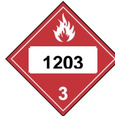
*A dangerous goods placard. The hazard class is (3) Flammable liquid, and the U.N. number 1203 identifies the material being hauled is gasoline or gasohol.*
