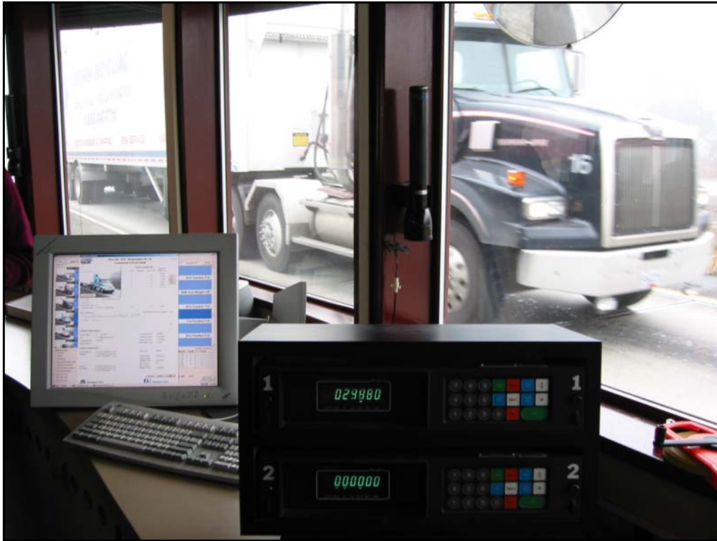
Figure 2-5. Truck Automatically Weighed Using the CVISN System at Bow Hill.
